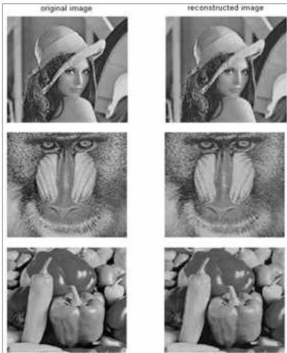
Figure 21. Original and Reconstructed Images Made by 3-FA-PSO Algorithm for Codebook with Size of 256
